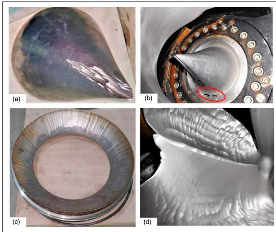
**Figure 1.** Eroded components of Pelton turbine of high head Kashang HPP (a, b) Needle, (c) Nozzle, (d) Bucket.
